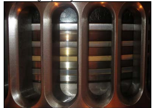
Excellent piston ring condition with minimal carbon deposits
